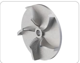
Anti-clogging impeller design passes soft debris <5mm, hard particles <1mm
