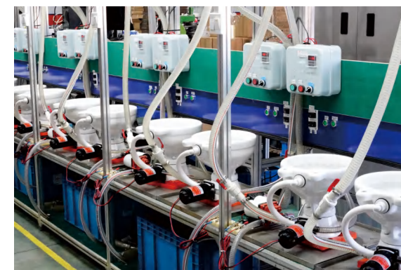
Toilet Lifespan Test Bench
